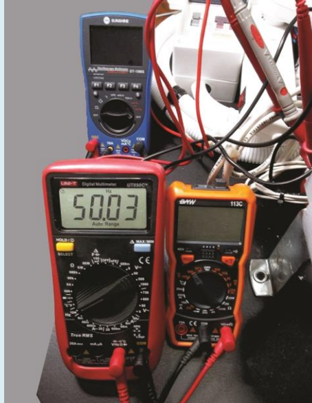
Figura 16. Vista del frecuencímetro encendido indicando los 50 (Hertz) de la corriente alterna (AC), junto al multímetro digital (voltímetro) apagado. Figure 16. View of the frequency meter turned on indicating the 50 (Hertz) of the alternating current (AC), next to the digital multimeter (voltmeter) turned off.
