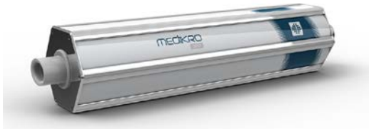
Figure 7. Calibrated 3L syringe used in performance tests.
