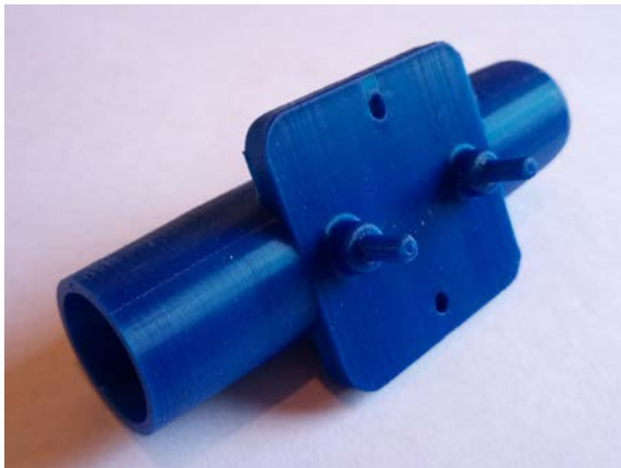
Figure 5. Finishing of the 3D printed Venturi tube.
