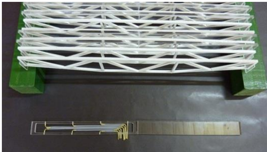
Fig. 7 Close view to the radar model and a panel with pressure taps. These are located on the front and rear of each panel
