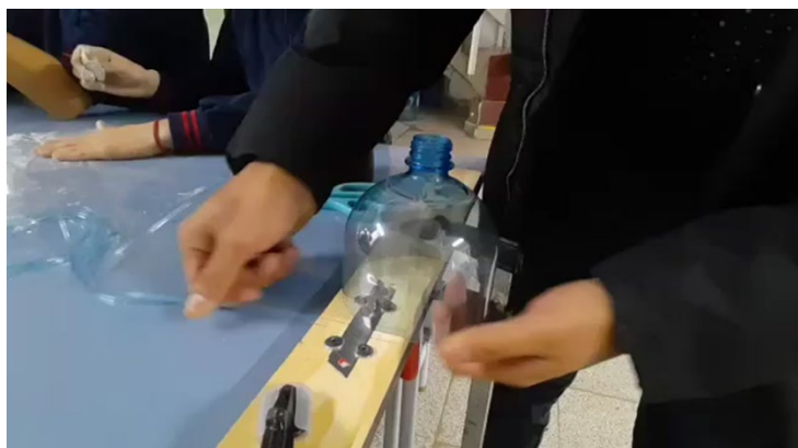
Figura 9. Obtención de hilos a partir de botellas de PET. Figure 9. Obtaining threads from PET bottles.
