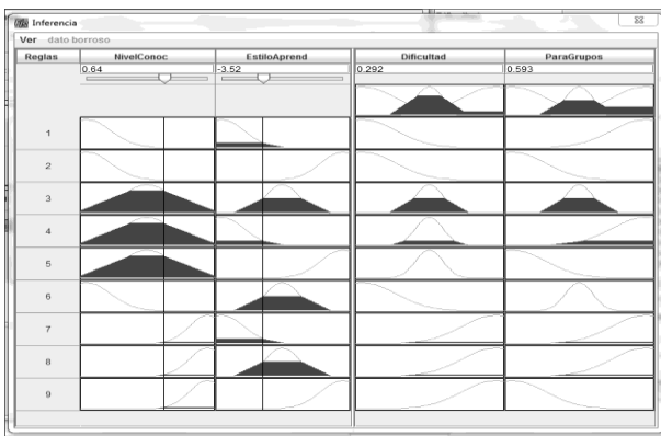
Fig. 5. Inference example where NivelConoc is strongly intermediate (0.64) and EstiloAprend is active and balanced in medium and equal manner (-3.52) implies that Dificultad is medium and high in medium and equal mode (0.292) and ParaGrupos is strongly group (0.593).
