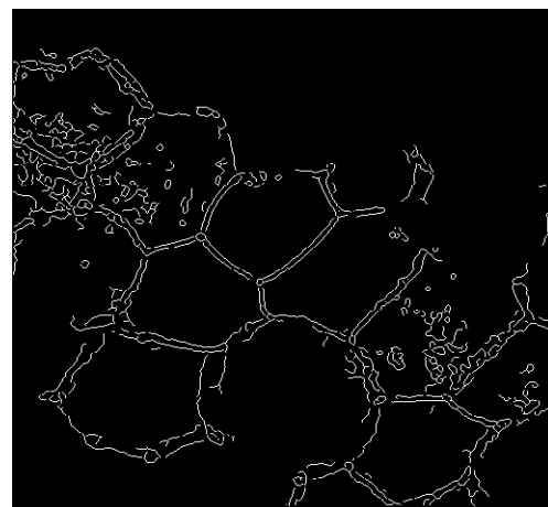
Fig. 5. (a) Border detection in Fig. 4(a) using border extraction after a median filtering, and (b) using the optimal Canny operator.
