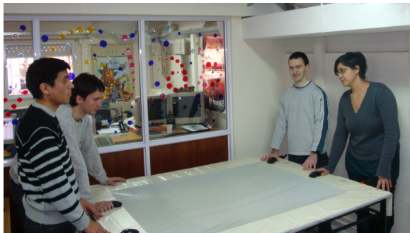
Fig. 1. Arrangement of the table surface. Each user is provided with a mouse and the surface image is displayed with the help of a projector.
